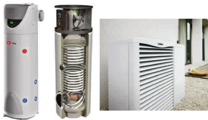
Figure 24: Left: Air/water heat pump: The outer part of the split unit. Inner part with buffer storage and hydraulic control system; up to 63°C (Photo: Vaillant Schweiz GmbH), Middle: Air/water heat pump boiler (energy source air). Outdoor air or indoor air with duct system. Built-in heat exchanger for solar or other energy sources. (Photo: Cipag AG), The picture shows a section through a hot water heat pump (boiler): At the top, the air is sucked in with the fan through the evaporator. In the middle, there is the heating coil, which transfers the heat to the drinking water, as well as the condenser at the bottom. Right: Outdoor unit of a split-system hot water heat pump.
